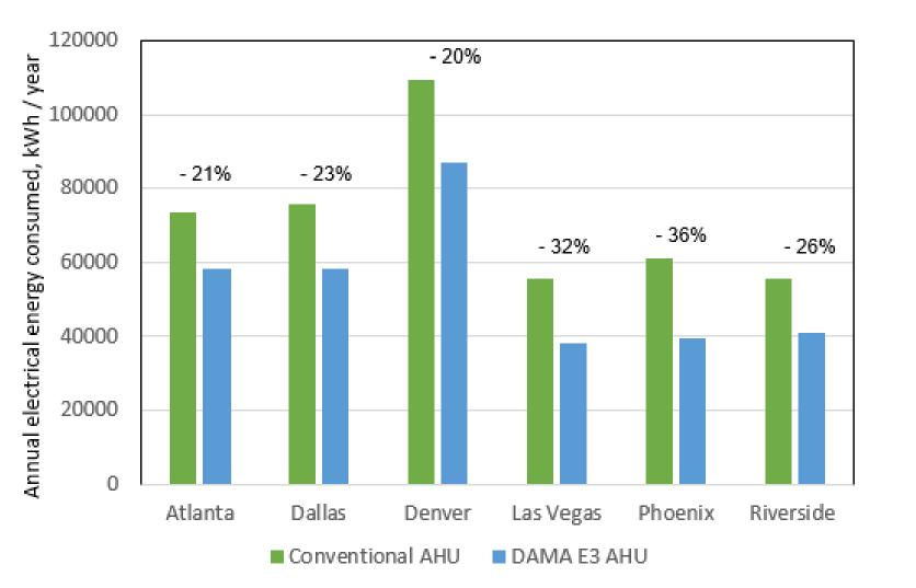
Indirect Evaporative Cooling-based Hybrid AHU
